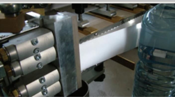
Special glue dosage system in case of particular customer requirements.
