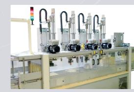
Enclosed polishing space with overhead polishing spindles
