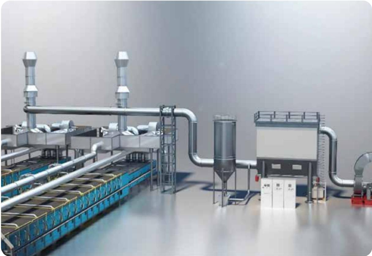
These include, for example, **bag filters for the capture of inorganic pollutants (so-called acid gases) and regenerative thermal oxidizers (RTO) to abate the VOCs that come from organic solvents** (and are responsible for bad odors).
