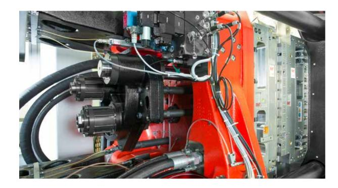
The toggle system and moving platen that make up the mould clamping unit have been designed using FEM structural analysis to optimise mechanical inertia and ensure excellent resistance to mechanical stress.
